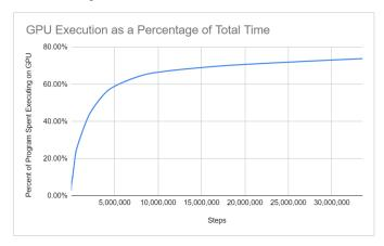
This result is surprising as we expect the GPU execution percentage to eventually decrease as the final summation cost increases. Additional testing could be performed to determine if the final summation eventually dominates the process' runtime.
